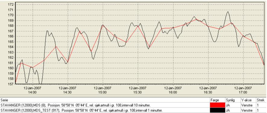
The 1 minute data are an average of 1 second samples for 60 seconds.
